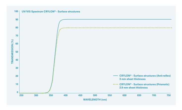
LT = Light transmission (Figures apply to 3 mm sheet thickness only.)
